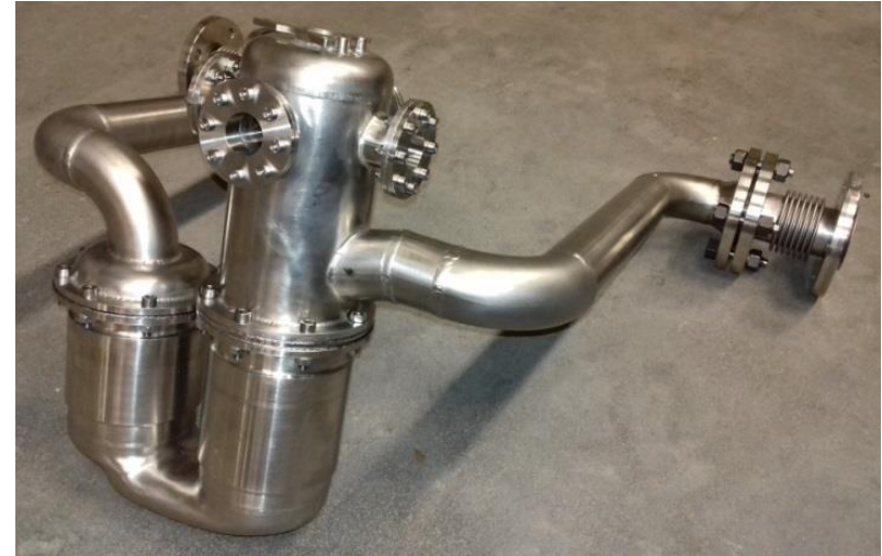
Optically accessible prototype of ammonia generator
