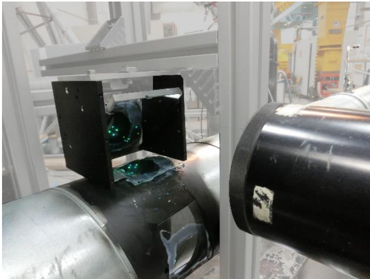
Velocity measurements with laser doppler anemometry
